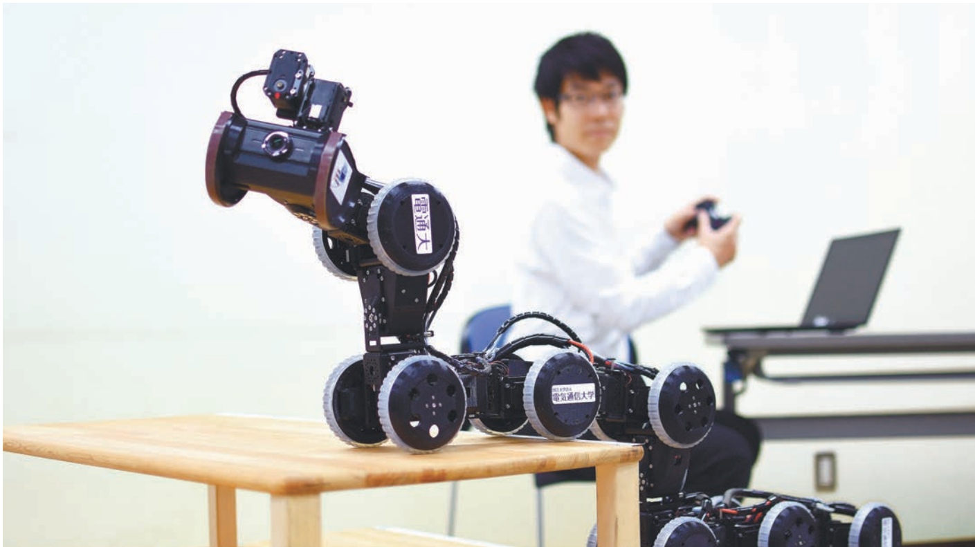
An older version of the snake-shaped robot, capable of climbing stairways and scale meter-high barriers. UEC
